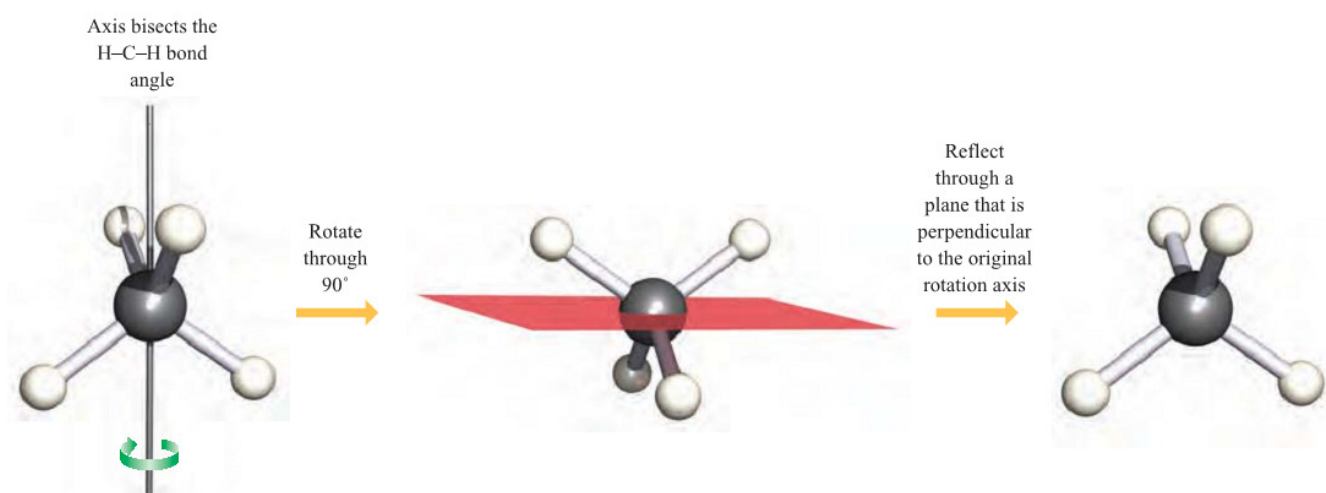
Figure 7: An improper rotation (or rotation–reflection), S_n , involves rotation about \frac{360^\circ}{n} followed by reflection through a plane that is perpendicular to the rotation axis. The diagram illustrates the operation about one of the S_4 axes in \text{CH}_4 ; three S_4 operations are possible for the \text{CH}_4 molecule.
