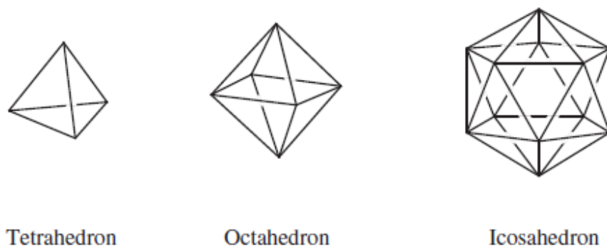
Figure 10: The tetrahedron ( T_d symmetry), octahedron ( O_h symmetry) and icosahedron ( I_h symmetry) possess four, six and twelve vertices respectively, and four, eight and twenty equilateral-triangular faces respectively.
